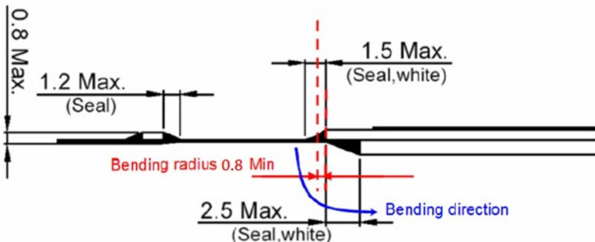
12.5 Avoid bending the film at IC bonding area. (>1.5mm)(this could damage the ILB bonding)
